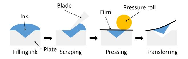
In this study, we investigated the effect of rheological properties of ink, printing speed and cell volume on the structure of the ink on the flat plate with graved cell. The dominant factor for appropriate gravure printing was clarified from the view point of rheological properties of TiO<sub>2</sub> ink.
